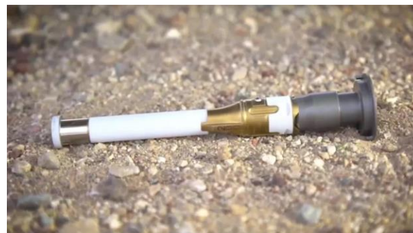
The rock samples are cached in titanium tubes. A collection of them will soon be dropped on the surface. (Image source: NASA/JPL-CALTECH/)
