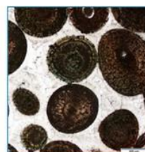
Grainstone: CaCO 3 grains >2mm self support (no mud support). Now the large pores filled with CaCO 3 cement.
