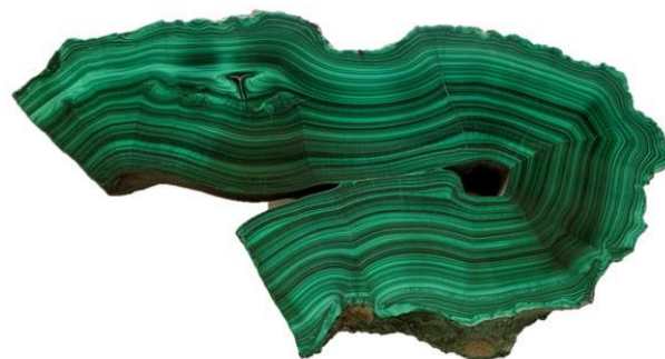
A beautiful, banded malachite Cu 2 (CO 3 )(OH) 2 coloured green by the essential copper in its composition. (© The Trustees of the Natural History Museum, London)
