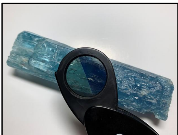
Aquamarine crystal from Vietnam. The dichroscope reveals the light blue and dark blue pleochroic colours of each 'ray', which combine to create the medium blue colour of this crystal. (© The Trustees of the Natural History Museum, London)
