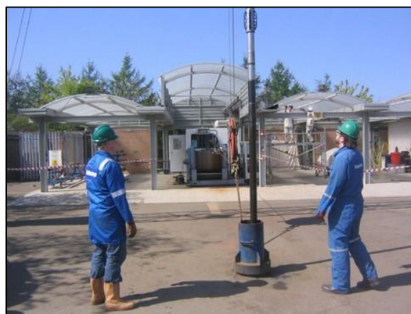
Figure 11: Wireline logging tool being "run-in hole". (Credit: Mike Millar)
