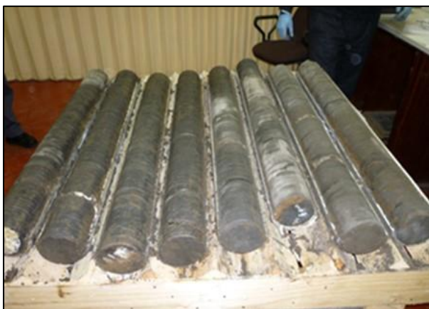
Figure 10: Conventional core laid-out in the laboratory prior to being described. (Credit: Mike Millar)
