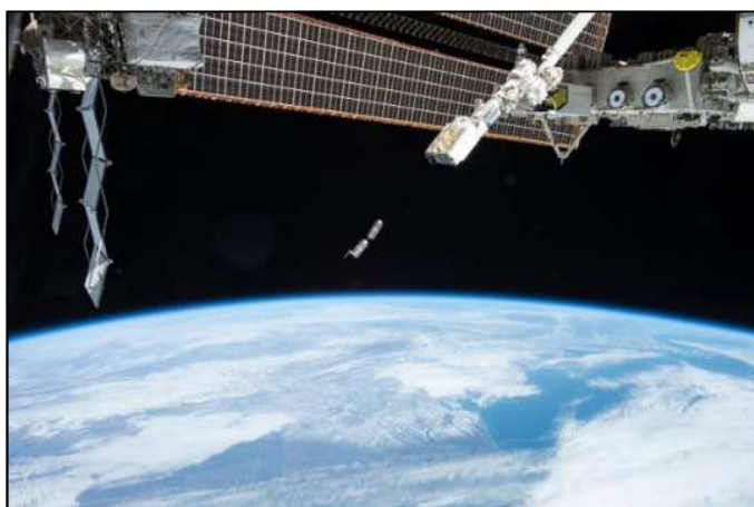
Fig. 4: Deployment of two of the QB50 CubeSats from the International Space Station
