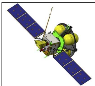
Fig. 10: SMILE in flight configuration (yellow tanks contain fuel needed to propel spacecraft into its highly elliptical Earth polar orbit).
