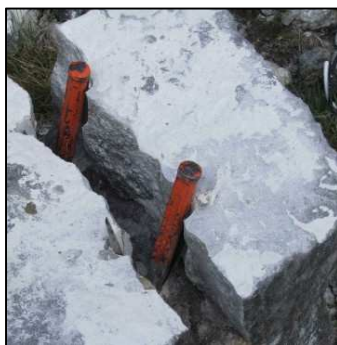
Fig. 2, 3: Plug and Feather Method – view & cross section
