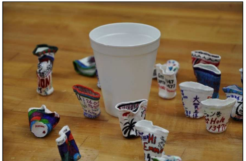
Fig. 5: 'Before and After' photo of Styrofoam Cups that were lowered to >3 km water depth at Shatsky – they shrank, and were then returned to the surface (Photo Credit: J. Prytulak)
