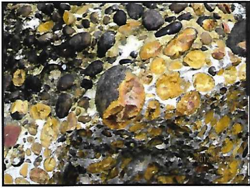
Fig. 1: Close-up of the HPS. Typical view of the HPS pebbles showing the black coating of the pebbles and the fracturing across the silica cement and siliceous pebbles as a coherent mass when broken. Scale: The large pebble is ca.6cm long.
