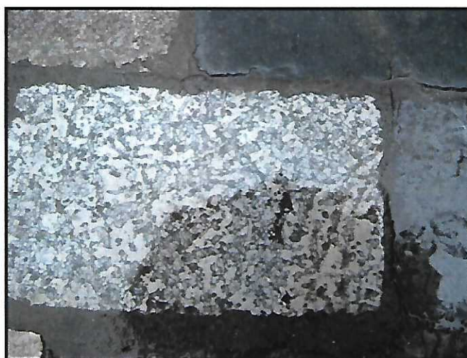
Fig. 4: Paving stones of another shallow water limestone showing bioturbation and possible stylolites and cementation features.
