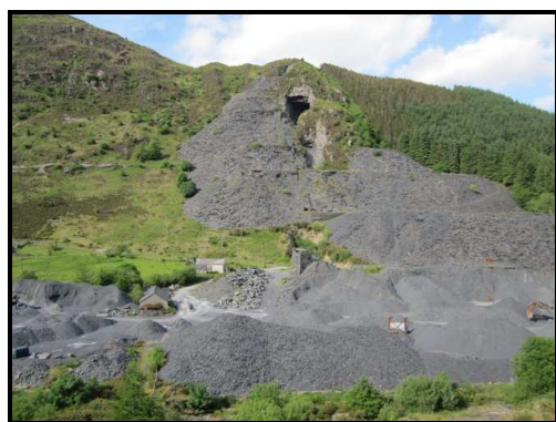
Fig. 3. Aberllefenni Slate Mine showing end-on exposure of the 'narrow vein' dipping at near 90°.
